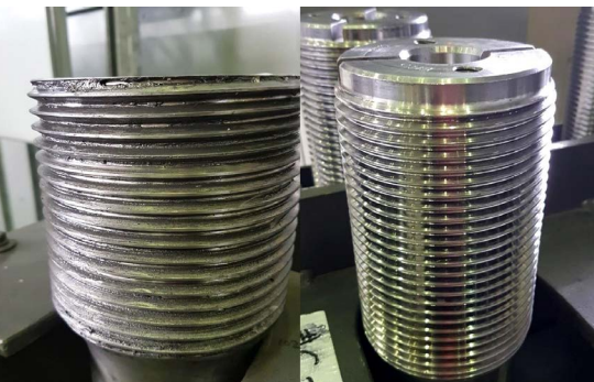
A removed bearing stud before and after cleaning.
